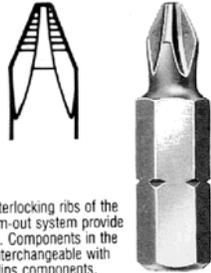
ACR®: The interlocking ribs of the ACR® anti-cam-out system provide higher torque. Components in the system are interchangeable with standard Phillips components.
