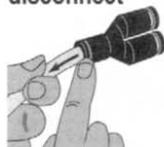
First depress the manual release button, then pull the tubing out of the fitting.
